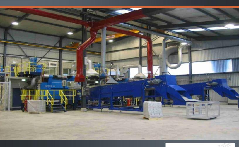
The project involved the development, planning, coordination, design, construction, and start-up of a magnesium alloy production and recycling facility using state-of-the-art magnesium metal melting and purification technology. The facility had a production capacity of 10,000 tonnes, producing of a variety of magnesium alloys.
